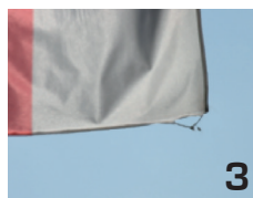
3 Damage along the seam extends to 3-5 cm to length.
